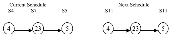
Figure 7. Current Schedule: node 4 is transmitting in the slot S4 , node 23 is transmitting in the slot S7 and node 5 is transmitting in the slot S5 . Node 4 reserves the slot S11 , in the current frame for the next frame, as XmtOp . This reservation takes place in the slot S4 . Node 4 transmits the updated schedule to its neighborhood. Node 23 is notified with the updated schedule. In the next slot, S5 , node 5 reserves the same slot S11 (selected randomly). Node 5 will be notified that this slot has already been reserved by another neighbor node (node 4) in the slot S7 by node 23. Node 5 will set its state in the slots S11 as state( S11 ) = Block_RX.
