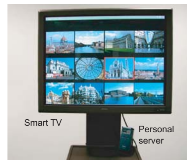
Figure 7. Smart TV executes PCL to access image data from personal server to display the GUI on its screen.
