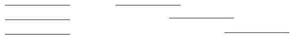
Figure A-1. Self aligning strings will either overlap completely (left) or overlap by some small, limited amount (right)
