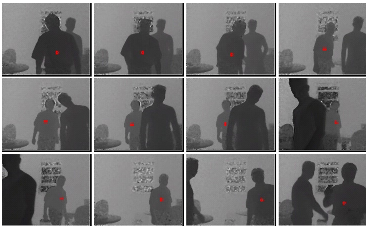
Figure 7. Tracking results of the proposed depth tracker in case of occlusion, scale and pose changes (frames 50, 57, 66, 80, 92, 99, 103, 122, 127, 141, 180, and 193)
