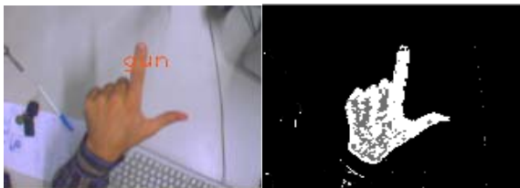
Figure 2. The image on the right is the result of the application of the skin color recognition scheme to the image on the left. Darker pixels correspond to lower probabilities of belonging to skin.
