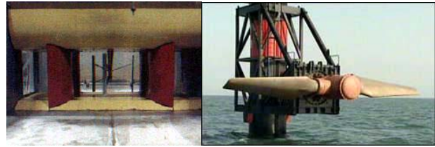
Figure 1 Vertical Axis Tidal Turbine (on left hand side, courtesy of Bluenergy) and Horizontal axis tidal turbine (on right hand side, courtesy of MCT)
