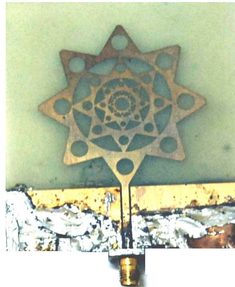
Figure 2. Photograph of the Wheel Shaped Fractal antenna
